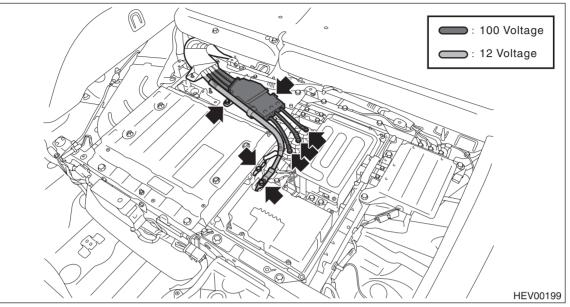
10) Remove the electric noise filter.
