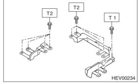
3) Install the inverter shield.
