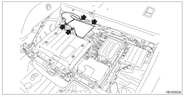
9) Remove the bolts and nuts and disconnect the ground terminal and the power cable.
