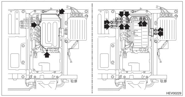
(3) Remove the bolts, and then remove the electric noise filter.
